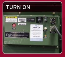
Operate these units by the onboard control or through a wired remote control that senses temperature where its located.
