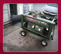
When low temperatures hit, the product stored in this container couldn't be allowed to freeze. Our unit was able to manage temperatures and with the thermostat inside the container the unit only ran when required, offering great fuel savings.
