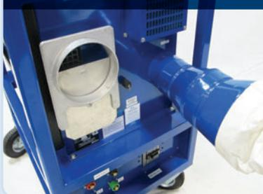
The warm, very humid re-activation air needs to be vented out of the space.
