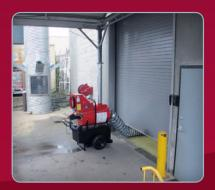
By placing the supply duct under the roll-up door, this warehouse was able to be heated with virtually zero time spent on prep or installation. The unit is highly mobile and easily moved if needed.
