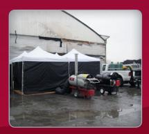
Highly mobile tent clusters on film locations are no problem for these self contained units. Large on-board fuel tanks allow the entire package to be rolled from site to site. All that is required is a standard 115 volt circuit.
