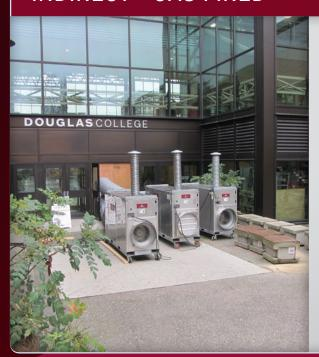
If you need major heat then this is the unit for you. Running on either propane or natural gas, they are great for heating construction sites or temporary structures. The fuel source can either be a large propane cylinder or a direct tie into a natural gas feed. Only clean, fresh air enters the space, as waste gases are vented up the flue pipe.
