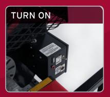
A selective toggle allows you to go from local ON/OFF control to a wired remote control.
