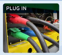
Convenient Cam-Lok connections make it easy to connect to 208 volt power and get the unit running fast.
