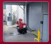
By placing the supply duct under the roll-up door, this warehouse was able to be heated with virtually zero time spent on prep or installation. The unit is highly mobile and easily moved if needed.
