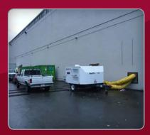
When cold temperatures hit and this warehouse's heating system failed, this quick response unit proved to be the ideal solution. Eliminating the delay in running power from within the building meant the relief was immediate.
