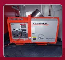
The onboard 7 kW generator is fed from the main fuel tank. It powers the unit and has two additional 15 Amp circuits for work lights, tools, etc.
