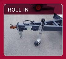
With a convenient trailer hitch, simply hook this unit up and roll it into your desired location.
