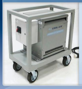
Packaged portable transformers allow you to step down from 600 volt to standard 208 volt power. They simply roll up to our equipment and plug in. Once the transformer is energized, throw the disconnect switch and you're ready to go.
