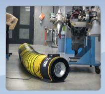
Electrical and machining work often creates unwanted heat and fumes. This ductable Black Max fan helped to expel this air by delivering it straight towards the building exhaust system.
