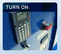
Simple ON/OFF control along with digital variable speed drive adjustment allows for complete unit control.
