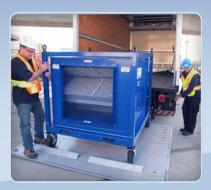
Large tires, forklift pockets, and lifting eyes make it a breeze to load this unit into any project.
