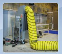
Equipped with powerful fans, these units can deliver air up to 75' away using our industrial supply air duct.
