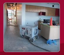
These electric furnaces are ideal for enclosed spaces where the unit must sit inside the space being heated. Safe, dry heat means that there is zero concern of toxic fumes.
