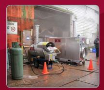
By ducting the warm air inside, direct heat can be provided where it is needed most. These units are weatherproof and designed to sit outside where combustion exhaust can vent safely away.
