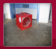
When spot heating was needed, this resistant heater provided ample heat in a lightweight, compact package.
