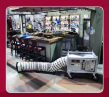
These electric furnaces are ideal for enclosed spaces where the unit must sit inside the space being heated. Safe, dry heat means that there is zero concern of toxic fumes.
