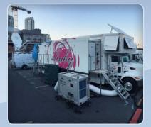
With the ability to supply air up to 100' away, this unit is perfect for when there is limited space inside the structure and the unit must sit outside. Return air duct can also be utilized when extra cooling or heating power is required.
