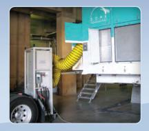
When this HD Broadcast truck lost half of its cooling, this 4 ton unit rolled in and seamlessly tied into the existing system.
