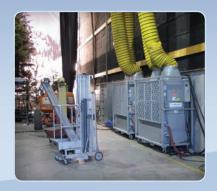
This production had a large amount of lights on their film set. By setting the units to one side and ducting the air to key areas we were able to achieve effective cooling.
