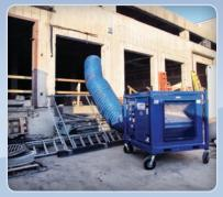
Construction sites often require extra ventilation during various stages of the project. This Hurricane was used to provide ample fresh air to workers inside while welding gases and exhaust fumes were present.
