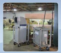
This large woodworking shop needed additional heating. Only 480 volt power was available and the electric furnace requires 208 volts. Problem solved with our portable transformer.
