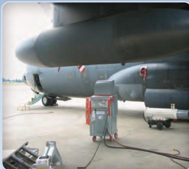
Specialized and adaptable, we were able to utilize this 3 ton unit to cool the cargo hold of this aircraft while technicians performed routine service.
