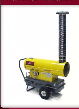
This compact indirect-fired diesel unit is ideal for smaller heating projects. Well equipped for remote locations, these units require a diesel fuel source and 115 volt power for the supply fan. Compact size and light weight allows for easy portability. Designed to sit outside with the supply air ducted inside, these units can also be positioned inside with the combustion gas ducted to the exterior.
