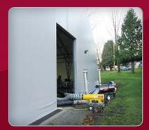
This steel storage building is utilized once a year for a large formal dinner/dance. The dedicated heating units didn't have sufficient heating strength when the evening festivities required suit, tie and formal dresses. The large heater from Cool Air provided the horsepower to get the temperature to comfortable levels while the quieter 27 kW unit kept the level maintained.
