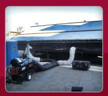
This temporary stage required a heat source to be located at the back of house to keep the artists from freezing. We were able to create a warm air bubble that allowed the talent to perform without their fingers falling off.
