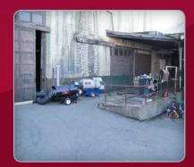
Film industry ready, these units delivered the warm air into this warehouse while the exhaust gases were vented straight from the machine located outdoors.
