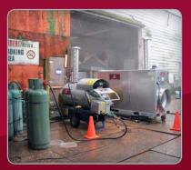
By ducting the warm air inside, direct heat can be provided where it is needed most. These units are weatherproof and designed to sit outside where combustion exhaust can vent safely away.
