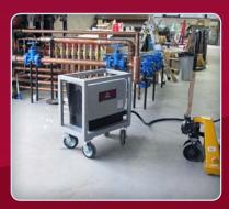
When the heater in this building was being replaced our 9 kW portable heater was used to maintain optimal temperatures in the work space. An unused range plug provided the power required and made for a simple and effective solution.
