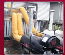
Ideal for applications where the heating equipment can sit outside. The heated air is delivered into the dwelling through insulated flex duct. The exhaust gases from the diesel or propane units are vented through the attached flue pipe.
