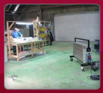
Working in large open spaces often means an uncomfortable environment. Rolling in this 14 kW radiant heater on our custom designed cart quickly heats things up and increases productivity.
