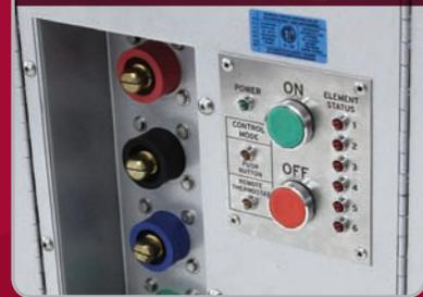
Controlled by either ON/OFF push buttons or our adjustable thermostat, these units allow for complete temperature control.
